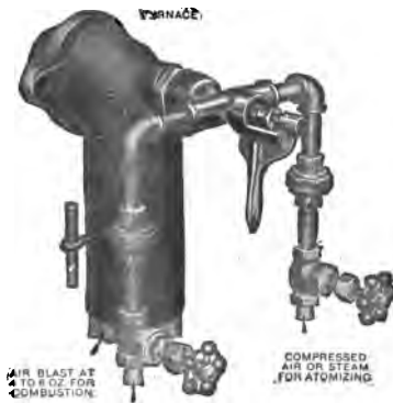
Fig. 199. Oil Burner with Air Blast and Compressed Air and Steam Connection for Atomizing Courtesy of Tate, Jones and Company, Pittsburgh, Pennsylvania
